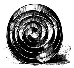
Drawing of ether chamber, with the bottom removed to shew the interior. The *volute*, of the same metal as the chamber, is soldered to the top, and reaches to one-sixteenth of an inch from the bottom.
