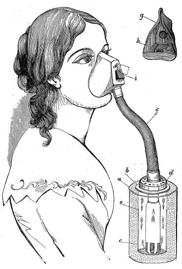
expiratory valve of the face-piece \* is made to move to one side, so as to leave uncovered more or less of the
