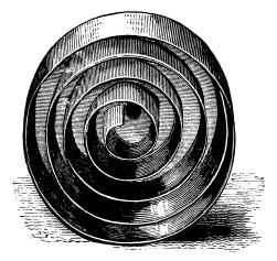
Drawing of ether chamber, with the bottom removed to shew the interior. The volute, of the same metal as the chamber, is soldered to the top, and reaches to one-sixteenth of an inch from the bottom.
