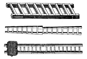
6th. Portable ladders for communicating with the boat from the ice, in cases where the current may have carried the body from the place at which it first sunk. These ladders may be *lengthened* by *unfolding* or *fitting* in, and made *buoyant* as may suit the occasion for which they are intended.
