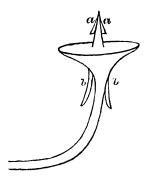
a a are barbs fitting with springs into mortices on the sides of the point.
