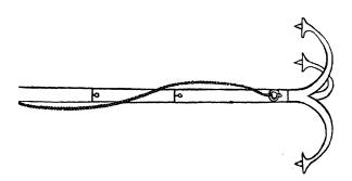
5th. An *Elongatable* grappling rod, which in cases where the body has sunk beneath the ice can be instantly adapted to any common depth of water, for the purpose of grappling for and bringing the sufferer to the surface.
